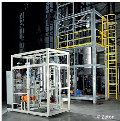
Industrial reference installation with HWAC-30 for purification of phosphoric acid at Solvay
