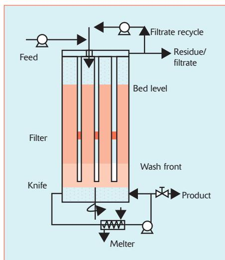
Figure 1 - TNO HWC in a melt crystallisation application
