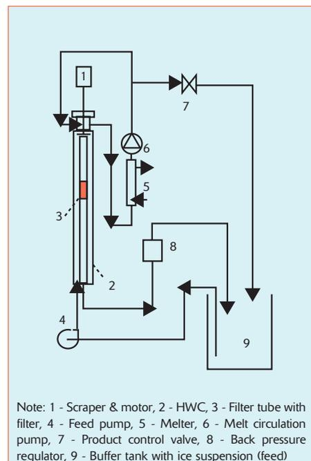
Note: 1 - Scraper & motor, 2 - HWC, 3 - Filter tube with filter, 4 - Feed pump, 5 - Melter, 6 - Melt circulation pump, 7 - Product control valve, 8 - Back pressure regulator, 9 - Buffer tank with ice suspension (feed)
