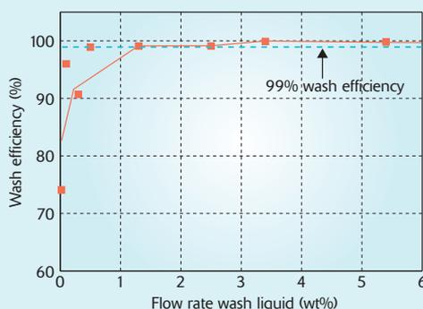
Note: The impurity to be removed was  $\text{SO}_4^{2-}$  and the applied wash liquid was a saturated NaCl solution
