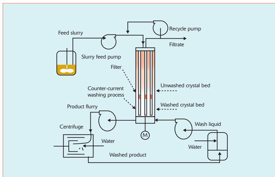
**Figure 3 - Layout of TNO HWC in a solvent switch application**
