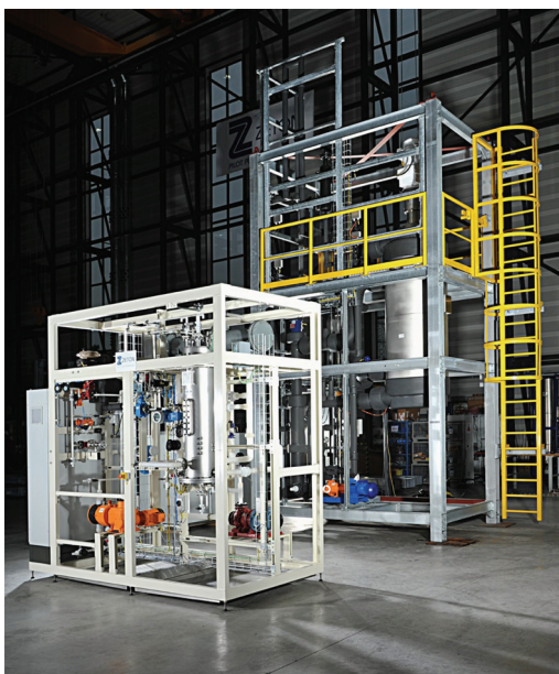
Example of an industrial scale melt crystallizer (back) and Hydraulic wash column (front)
